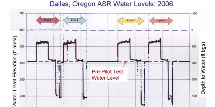
This Hydrograph illustrates water level changes in response to injection and recovery at the ASR well.
