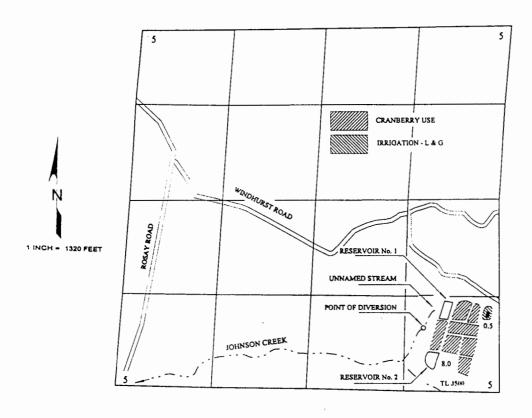
THE POINT OF DIVERSION IS LOCATED 900 FEET NORTH AND 1040 FEET WEST; AND RESERVOIR No. 1 IS LOCATED 1160 FEET NORTH AND 780 FEET WEST; AND RESERVOIR No. 2 IS LOCATED 410 FEET NORTH AND 1000 FEET WEST; ALL FROM THE SOUTHEAST CORNER OF SECTION 5, ALL WITHIN THE SE'ASE'A OF SECTION 5, TOWNSHIP 29 SOUTH, RANGE 14 WEST, W.M.; COOS COUNTY.
