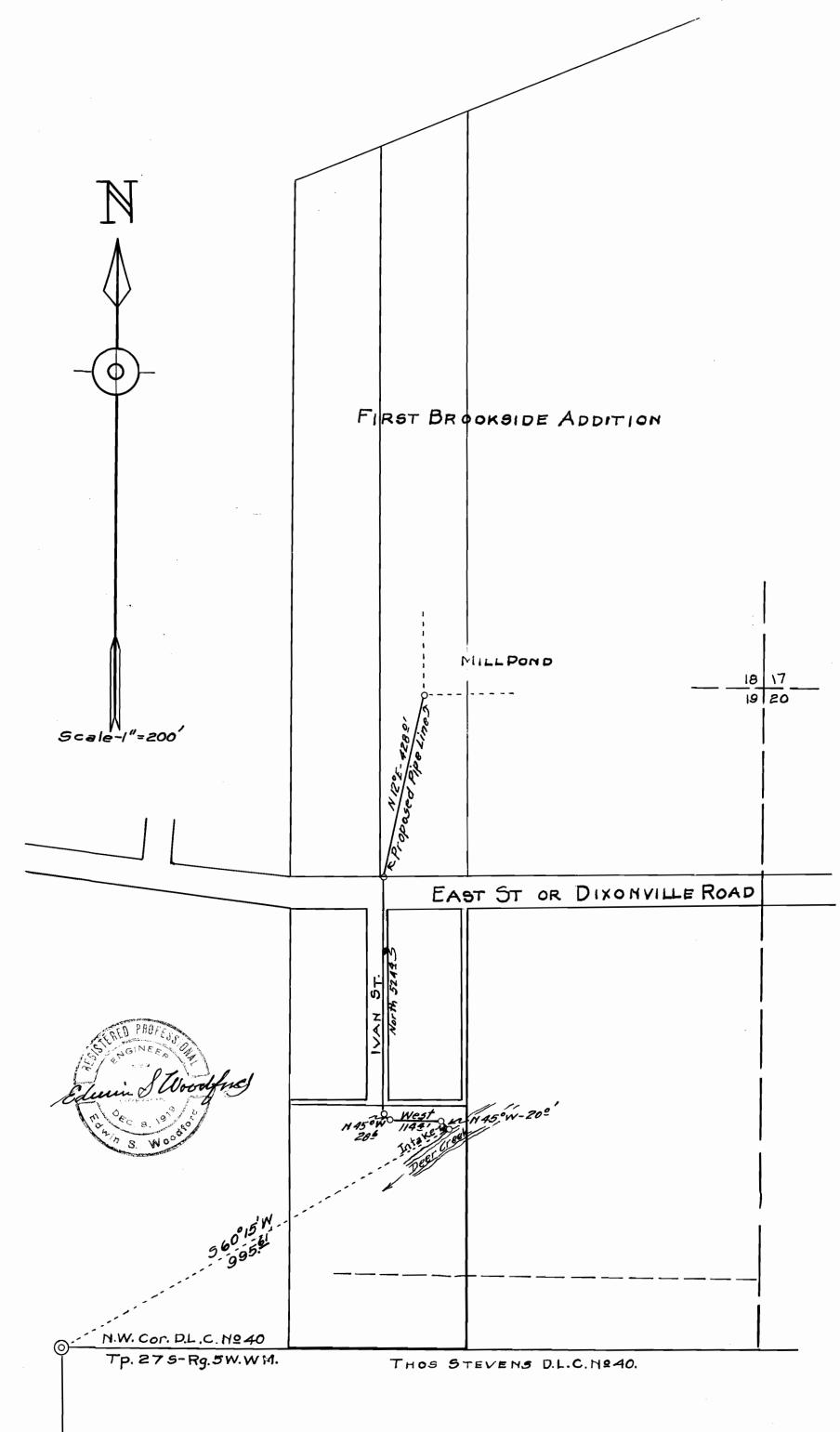
I Edwin 5 Woodford of Salem Oregon do hereby Certify that this map was made from notes taken during an actual survey made by me on July 31 1943 and that it correctly represents the works described in the accompanying application together with the location of streams and other ditches in the immediate vicinity.
