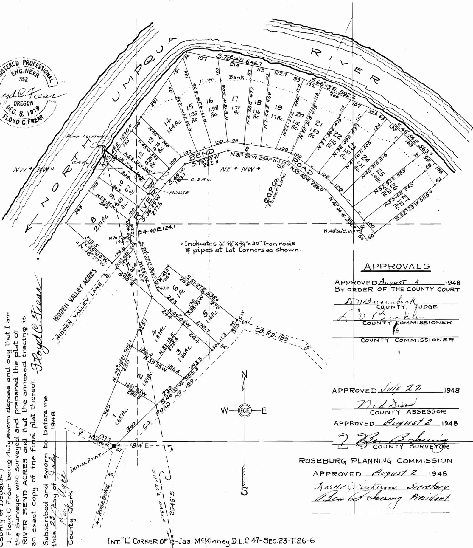
Indicates 1/2" 5/8" & 3/4" x 30" Iron rods & pipes at Lot Corners as shown.
