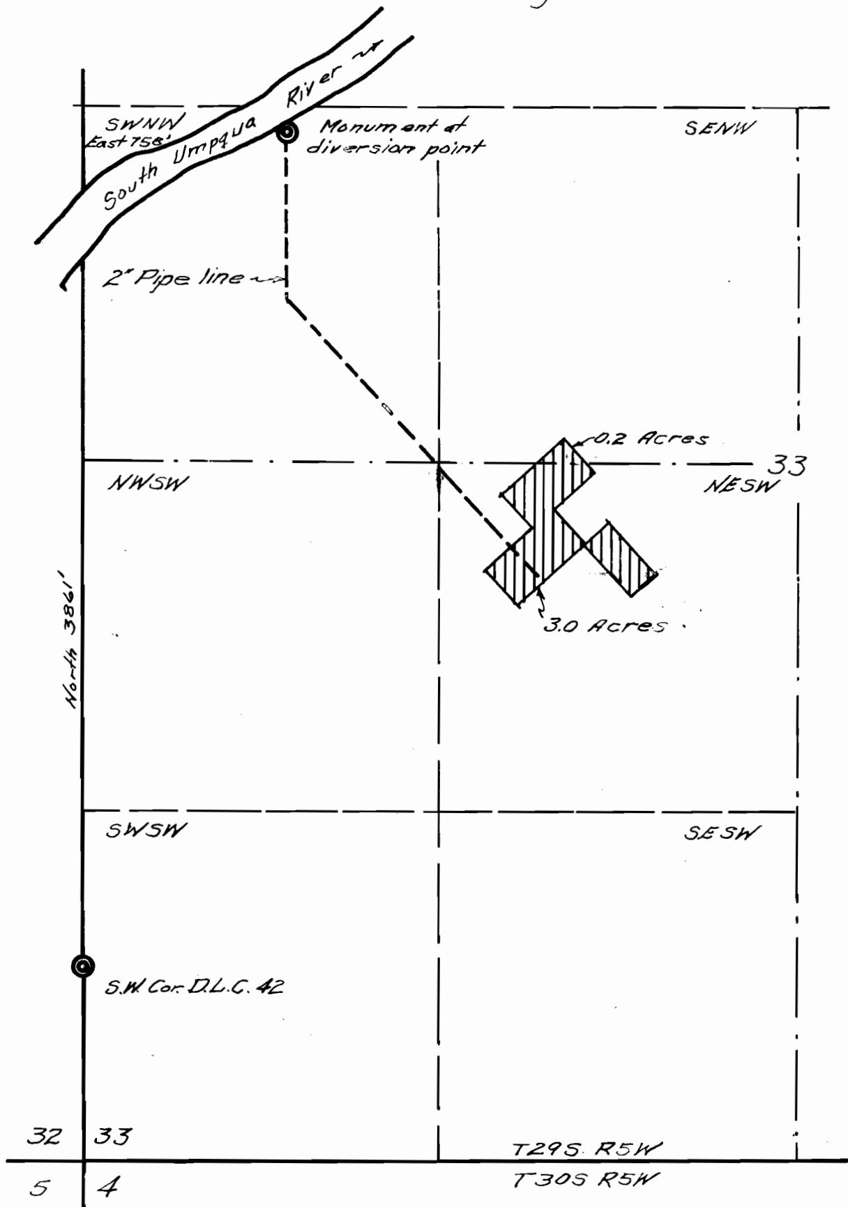
I, John H. Markham, Jr. of Riddle, Oregon do hereby certify that this map was made from notes taken during an actual survey made by me on Aug. 23, 1951, that the monument shown on this map consisting of a 1x30" iron pipe driven 24" in ground from which an Alder 11" in diam. bears S49°E 7.0' dist. mkd. W.R. 2880 B.T. An Ash 24" diam. bears, S14°W 6.5' dist. mkd. W.R. 2880 B.T. The monument is North 3861.0' and East 758.0' from the S.W. corner of Section 33, T29S, R5W, W.M. Douglas County, Oregon.
