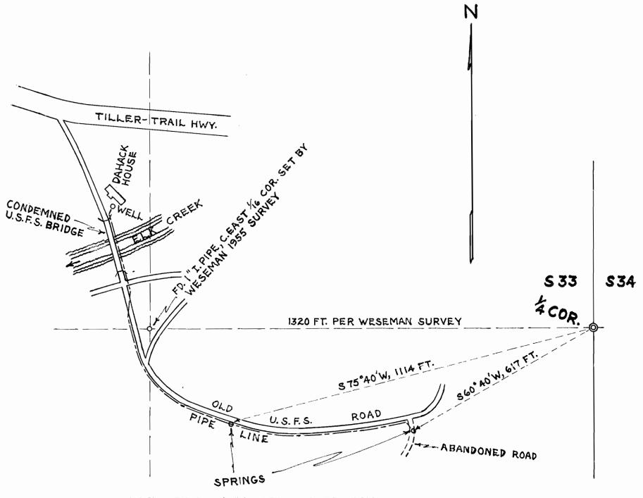
NOTE: PIPE LINE TO CARRY WATER FROM SPRINGS TO DAHACK WELL
