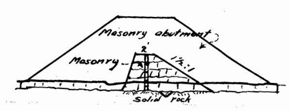
SECTION OF SPILLWAY Note - Masonry weir not constructed as yet Dec. 1919. To be broken by flashboard weir.
