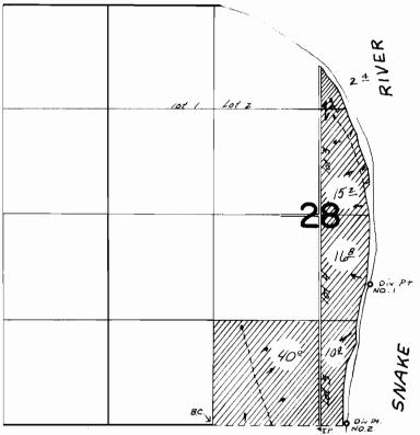
Div Pt No. 1 located 1760N + 1960'E; Div Pt No. 2 located 20' N. +1660'E; from SE Cor 5W'4 SW'4 Sec 28
