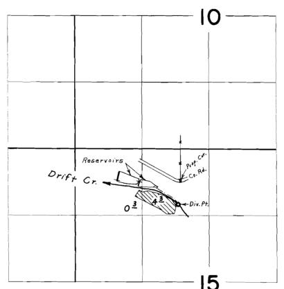
Div. Pts. located: Stream, 373'S. & 2030'E.; Reservoir, 3260'S & 830'E.; 3280'S. & 1270'E. all from W. & Corner Sec. 10
