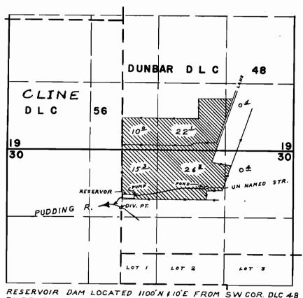
RESERVOIR DAM LOCATED HOO'N FIO'E FROM SW COR. DLC 48 RIVER DIV. PT. LOCATED 890'N & 10'W FROM SW COR DLC 48
