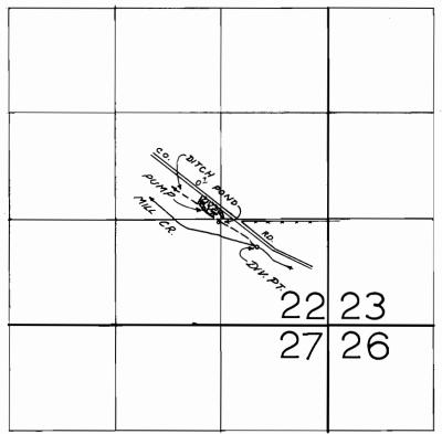
PUMP LOCATED 175'W É 120'N FROM SE COR OF NW4 OF SE 4 OF SEC 22 POND LOCATED 50'W É 20'S FROM NE COR OF SW4 OF SE 4 OF SEC 22 DIV. PT. LOCATED 450'E É 320'S FROM NW COR. OF SE 14 OF SE 14 OF SEC 22
