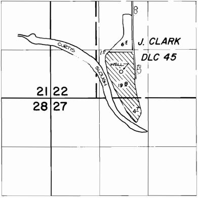
WELL IS LOCATED 700'N, AND 1910'E, FROM THE S.W. CORNER OF SECTION 22.
