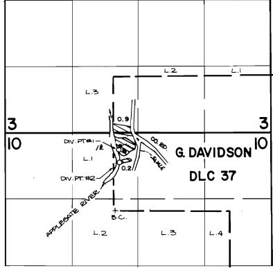
DV. PT. #1 IS LOCATED 350'S. AND 350'W.; DV. PT. #2 IS LOCATED \$50'S. AND 350'W.; BOTH FROM THE N. 1/4 CORNER. OF SECTION 10.
