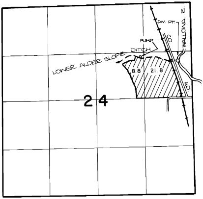
DIVERSION POINT IS LOCATED 1050' N. AND 350' W. FROM THE E.1/4 CORNER OF SECTION 32.
