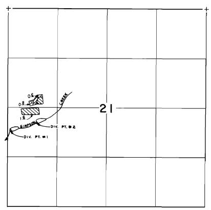
DIV. PT. #1 LOCATED 610'S. \$ 80'E. FROM W. 1/4 CORNER SECTION 21 DIV. PT. #2 LOCATED 400'S. \$ 775'E. FROM W. 1/4 CORNER SECTION 21
