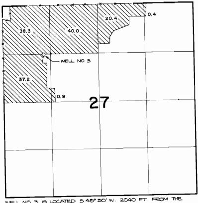
WELL NO.3 IS LOCATED S 48° 30' W. 2040 FT. FROM THE N.1/4 CORNER OF SECTION 27.
