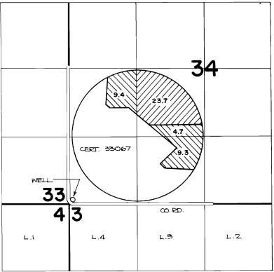
THE WELL IS LOCATED 80 FT. N. AND 50 FT. E. FROM THE S.W. CORNER OF SECTION 34.
