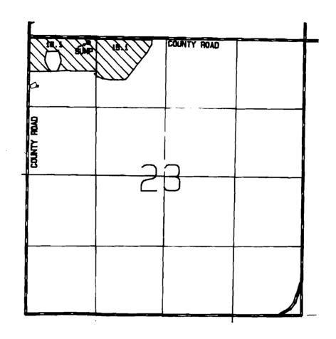
SCALE: 1" = 1320 SUMP LOCATED 120 FT. S. AND 1150 FT. E. FROM NW COR. SEC. 23
