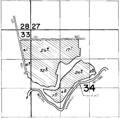
THE DIVERSION POINT IS LOCATED 2390'S. AND 2220'E. FROM THE N.W. CORNER OF SECTION 34.
