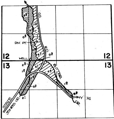
DIVERSION POINT IS LOCATED 360'S. AND 1450'E. FROM THE N.W. CORNER OF THE S.W. 1/4 S.W. 1/4 OF SECTION 12. WELL IS LOCATED 1190'S. AND 1350'E. FROM THE N.W. CORNER OF THE S.W. 1/4 SW. 1/4 OF SECTION 12.
