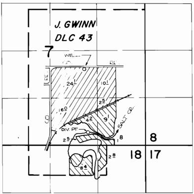
THE WELL IS LOCATED 2140 N. AND 1710 W., AND THE DIVERSION POINT IS LOCATED 350 N. AND 1600 W., BOTH FROM THE S.E. CORNER OF SECTION 7.
