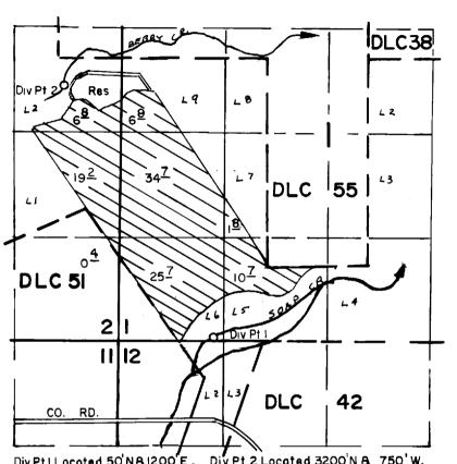
Div Pt I Located 50'N& 1200'E, Div Pt 2 Located 3200'N & 750'W, Both From The SW Corner Section 1.
