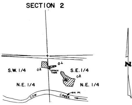
DIV. PT. LOCATED 560' S. C 290' E. FROM N.E. I/IS CORNER SECTION 2
