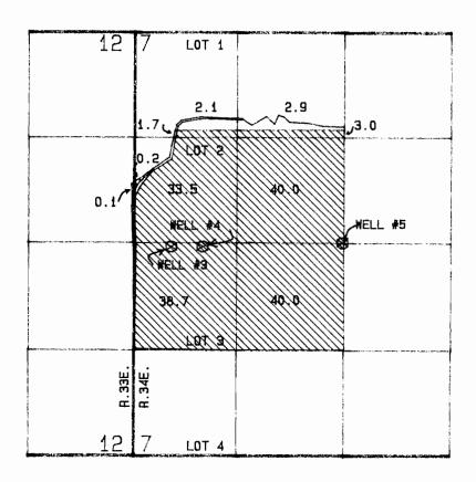
WELLS LOCATED: WELL 3 - 40 FT SOUTH AND 450 FT EAST; WELL 4 - 30 FT SOUTH AND 840 FT EAST; WELL 5 - 30 FT NORTH AND 2570 FT EAST; ALL FROM THE WEST 1/4 CORNER SECTION 7.
