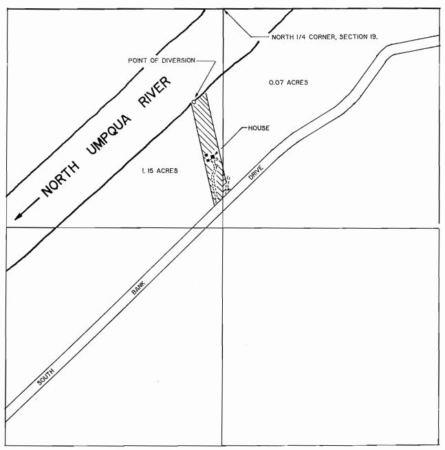
THE POINT OF DIVERSION IS LOCATED 760 FEET NORTH AND 190 FEET WEST FROM THE SOUTHEAST CORNER OF THE NEI/4 NWI/4 OF SECTION 19, BEING WITHIN THE NEI/4 NWI/4 OF SECTION 19, TOWNSHIP 26 SOUTH, RANGE 4 WEST, W. M.
