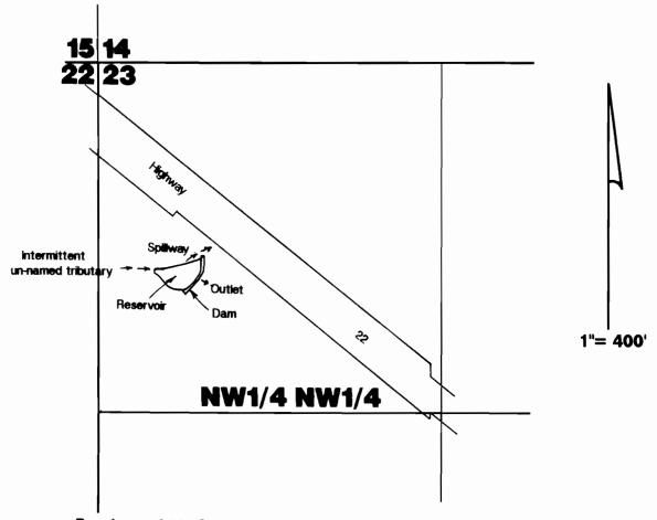
Dam located 800'S and 390'E from NW Corner Section 23.
