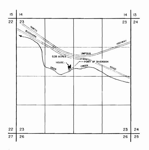
THE POINT OF DIVERSION IS LOCATED 290 FEET NORTH AND 2800 FEET WEST FROM THE EAST I/4 CORNER OF SECTION 23, BEING WITHIN THE SE I/4 OF THE NW I/4 OF SECTION 23 TOWNSHIP 27 SOUTH, RANGE 5 WEST, W.M.
