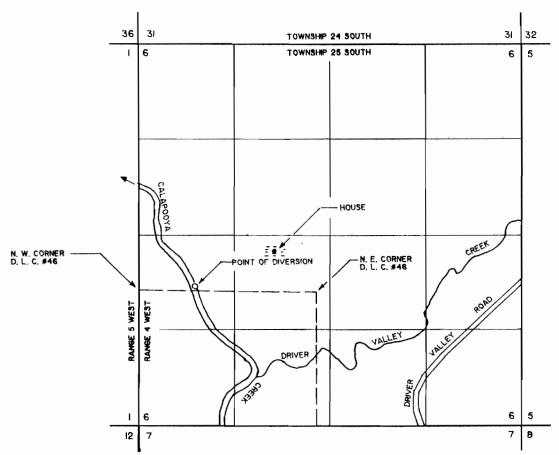
THE POINT OF DIVERSION IS LOCATED 3340 FEET SOUTH AND 1860 FEET WEST FROM THE NORTH 1/4 CORNER OF SECTION 6, BEING WITHIN THE NW1/4 OF THE SW1/4 OF SECTION 6, TOWNSHIP 25 SOUTH, RANGE 4 WEST, W. M.
