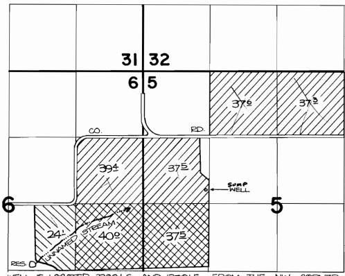
WELL IS LOCATED 2380'S. AND 1250'E. FROM THE NW. CORNER OF SECTION 5. THE DIVERSION POINT FOR THE RESERVOIR IS LOCATED 3810'S. AND 2190'W. FROM THE N.W. CORNER OF SECTION 5.
