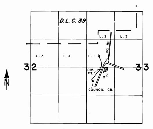
DIVERSION POINT LOCATED 60' S. & 640' E. FROM W. 1/4 CORNER SECTION 33.
