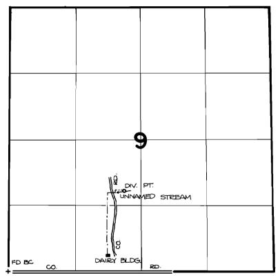
DIVERSION POINT IS LOCATED 1610' N. AND 2300' F. FROM THE S.W. CORNER OF SECTION 9
