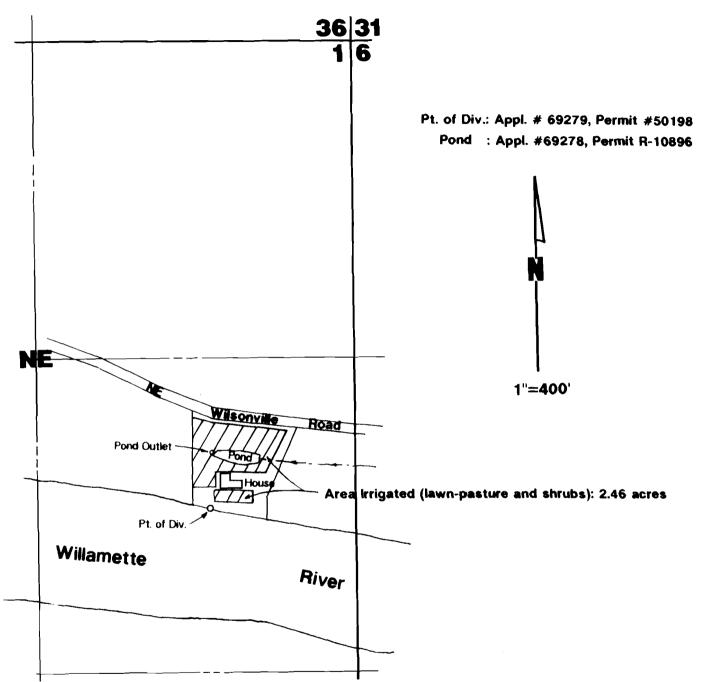
Pt. of Div. 1950'S and 600'W from NE Corner Section 1. Pond Outlet 1715'S and 590'W from NE Corner Section 1.
