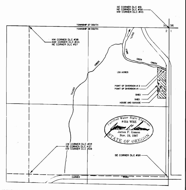
POINT OF DIVERSION # I IS LOCATED 680 FEET SOUTH AND 50 FEET WEST. POINT OF DIVERSION #2 IS LOCATED 660 FEET SOUTH AND 100 FEET WEST, BOTH FROM THE NORTHEAST CORNER OF SECTION 7, AND BOTH BEING WITHIN THE NORTHEAST 1/4 OF THE NORTHEAST LIVE TO THE LOCATION OF PROPERTY OWNERSHIP BOUNDARY LINES.
