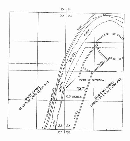
THE POINT OF DIVERSION IS LOCATED 1770 FEET NORTH AND 90 FEET WEST FROM THE SOUTHEAST CORNER OF SECTION 22, BEING WITHIN THE NE 1/4 OF THE SW 1/4 OF SECTION 22, TOWNSHIP 26 SOUTH, RANGE 6 WEST, W.M., DOUGLAS COUNTY.
