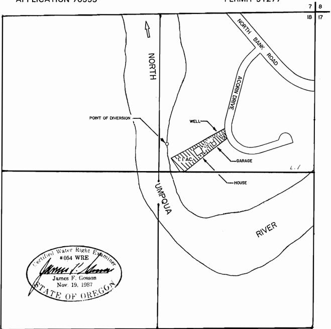
THE POINT OF DIVERSION IS LOCATED 1080 FEET SOUTH AND 1250 FEET WEST FROM THE NORTHEAST CORNER OF SECTION 18, BEING WITHIN THE NE 1/4 OF THE NE 1/4 OF SECTION 18, TOWNSHIP 28 SOUTH, RANGE 4 WEST, W.M., DOUGLAS COUNTY.
