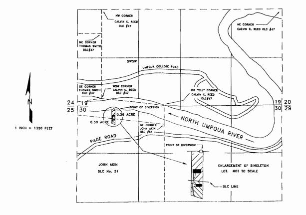
THE POINT OF DIVERSION IS LOCATED 320 FEET SOUTH AND 360 FEET EAST FROM THE WSW CORNER OF CALVIN C. REED DLC #47, BEING WITHIN THE NW%NW% OF SECTION 30, TOWNSHIP 26 SOUTH, RANGE 5 WEST, W.M., DOUGLAS COUNTY.
