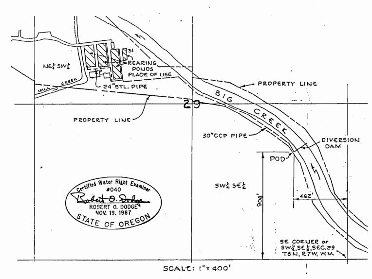
POD LOCATED 908 NORTH AND 462 WEST OF THE SE CORNER OF THE 5W \$ SE & OF SECTION 29
