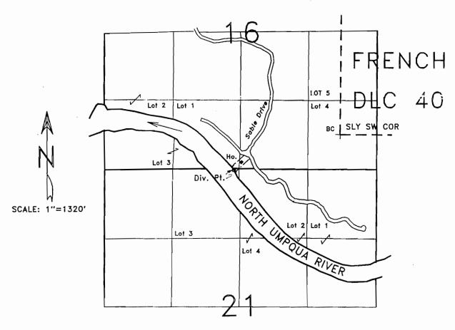
Div. Pt. is located /10' S. & 2050' W. from S'ly SW corner of DLC 40.
