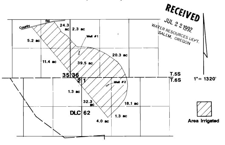
Well #1 located 1050'N &380'E from SW corner Section 36.
