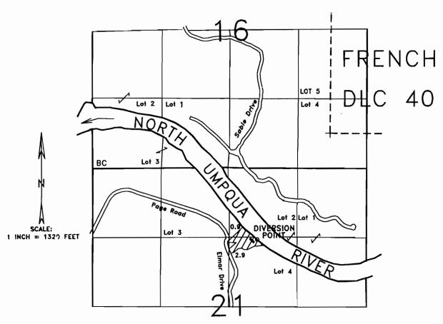
DIVERSION POINT IS LOCATED 1380'S. & 3160'E. FROM NW COR. SEC. 21.
