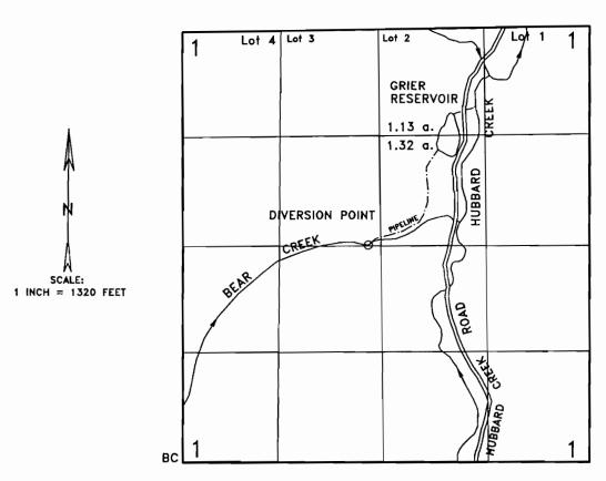
DIVERSION POINT IS 2660' N. & 2310' E. FROM SW COR. SECTION 1.
