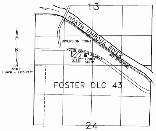
DIVERSION POINT IS LOCATED 1200 FEET NORTH AND 2580 FEET WEST FROM THE SOUTHEAST CORNER OF SECTION 13.
