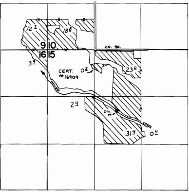
DIVERSION POINT LOCATED 1720'S & 680'W FROM THE N 14 COR. SECTION 15
