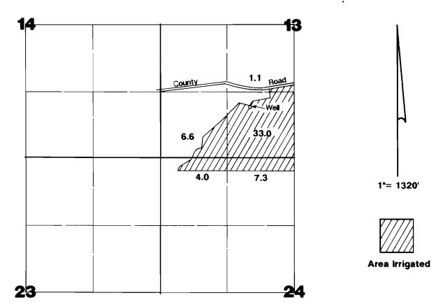
Well located 1030'N & 1760'E from SW corner of Section 13.
