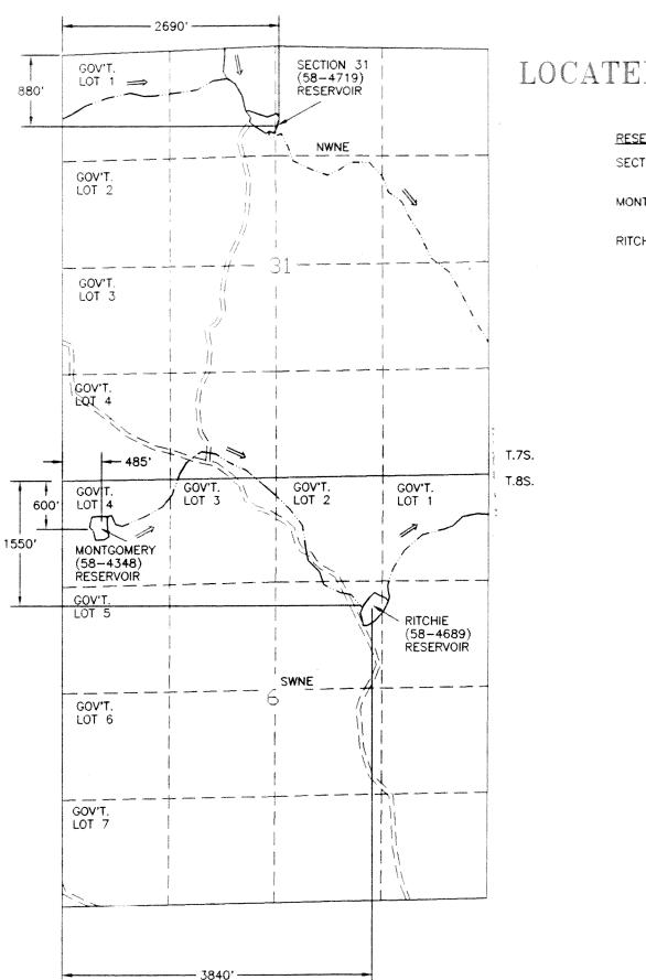
RESERVOIR & JDR NO. LEGAL DESCRIPTION LAT. & LONG. APP. NO. N: 44°55'01.4" SECTION 31 (58-4719) RESERVOIR NW1/4 NE1/4 SECTION 31 R-78274 W: 117'44'15.8" T.75., R.41E., W.M. MONTGOMERY (58-4348) RESERVOIR GOV'T. LOT 4, SECTION 6, N: 44"54'12.3" R-78276 T.8S., R.41E., W.M. W: 117'44'41.7" RITCHIE (58-4689) RESERVOIR SW1/4 NE1/4, SECTION 6 N: 44\*54'06.3" R-78275 T.8S., R.41E., W.M. W: 117'43'53.5"
