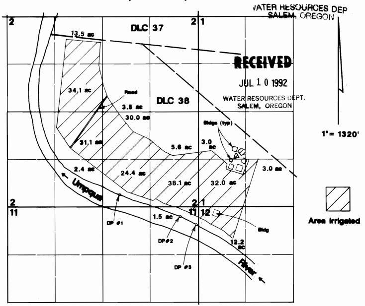
Div Pt #1 located 324.45'N & 2164.25'W to corner common to Sections 1, 2, 11 & 12. Div Pt #2 located 251.99'S & 476.49'W from corner common to Sections 1, 2, 11 & 12. Div Pt #3 located 447.5'S & 37.5'W from corner common to Sections 1, 2, 11 & 12.
