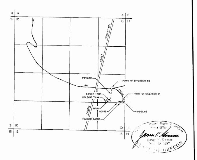
POINT OF DIVERSION #1 IS LOCATED 1180 FEET SOUTH AND 80 FEET WEST FROM THE EAST 1/4 CORNER OF SECTION 10. POINT OF DIVERSION #2 IS LOCATED 630 FEET SOUTH AND 660 FEET WEST, BOTH POINTS OF DIVERSION BEING WITHIN THE NORTHEAST 1/4 OF THE SOUTHEAST 1/4 OF SECTION 10, TOWNSHIP 31 SOUTH, RANGE 15 WEST, W.M., COOS COUNTY.
