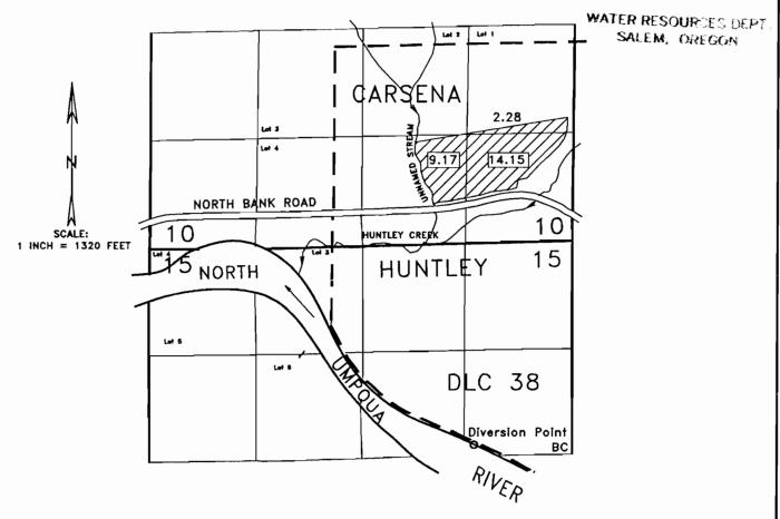
DIVERSION POINT IS LOCATED 150' N. & 1180' W. FROM E1/4 CORNER OF SECTION 15.
