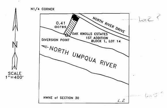
THE DIVERSION POINT IS LOCATED 320 FEET SOUTH AND 400 FEET EAST FROM THE NORTH 1/4 CORNER OF SECTION 30.
