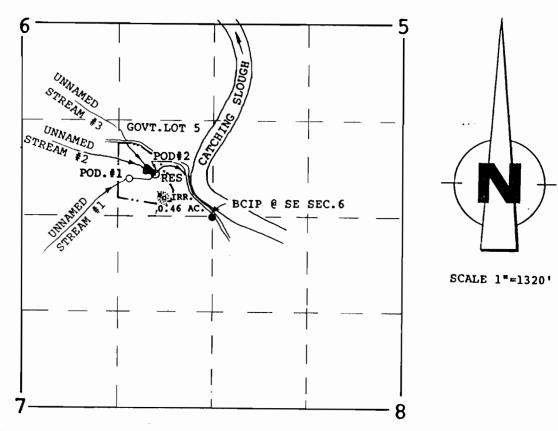
RESERVOIR LOCATED 583.5'N. AND 884.4'W.FROM SE COR.SEC.6 POD #1 LOCATED 515.1'N. AND 1072.3'W. FROM SE COR.SEC.6 POD #2 LOCATED 583.5'N. AND 884.4'W.FROM SE COR.SEC.6
